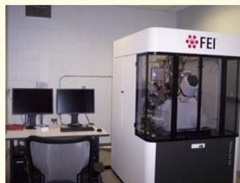
*The FEI Helios dual-beam FIB
