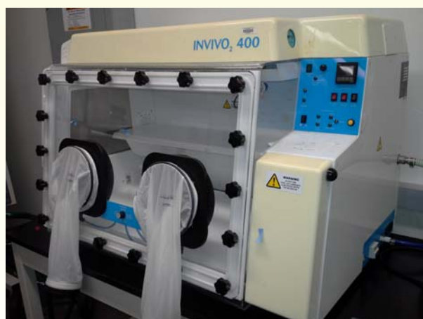
The InVivo bio glove box for culturing or handling anaerobic cells.
