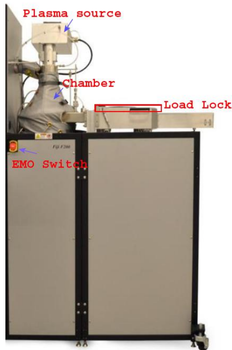
Fig 1. Main items of the Fiji ALD system.
